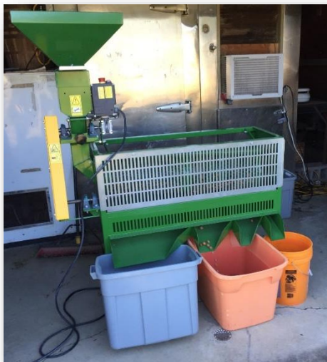
Italian-made size sorter and sheller at Rutgers (Chianchia P80 Super).
