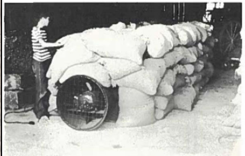
Fig. 2-A A small lot of grain being dried with a small fan. The duct in this case is the size of the fan outlet.
