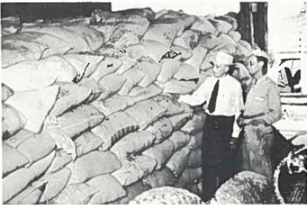
Fig. 1-A A large lot of wheat being dried with a hay drier fan. The fan is located just inside the barn door. The air duct inside the pile of bags is about 4 feet wide and 4 feet high. The depth of grain over the duct is the same as the width on each side of the duct.
